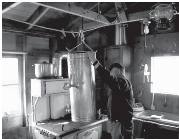
Art demonstrating his ceiling-mounted winch that he uses for lifting his filtering can.
